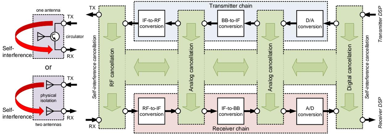
Fig. 2. Generic illustration of an inband full-duplex transceiver with various self-interference cancellation solutions.
