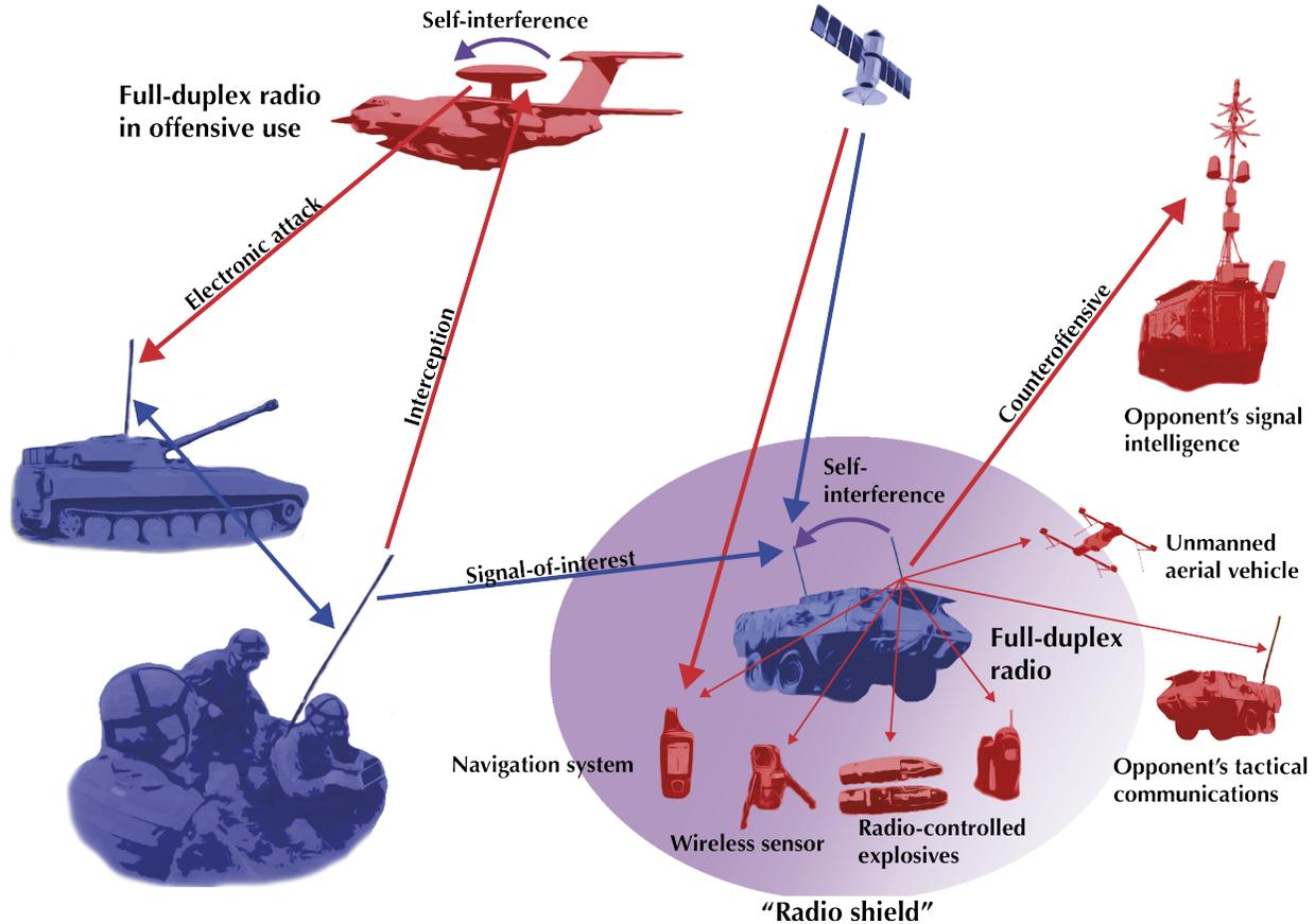
Fig. 1. Conceptual view of using inband full-duplex radio transceivers in tactical communications and electronic warfare.
