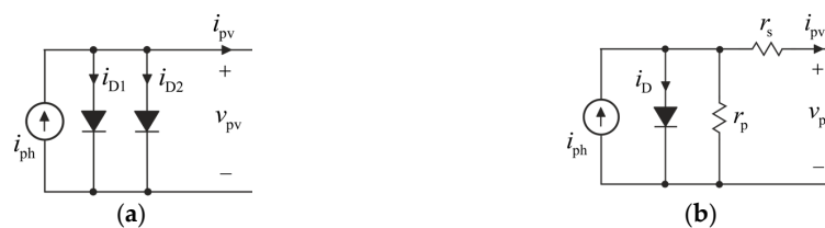
Figure 2. Equivalent circuits of a solar cell: (a) ideal two-diode model; and (b) practical single-diode model.
