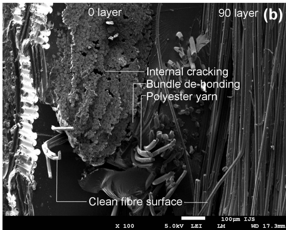
Fig 12: SEM images from tensile fracture surface of RS0-C composites
