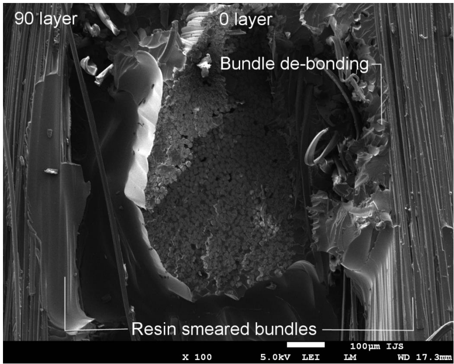
Fig 14: SEM images from tensile fracture surface of RS5-70-C composites
