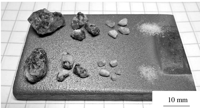
Fig. 6 Tested 355 MPa steel sample, and unused abrasives on upper row and the same after the test below
