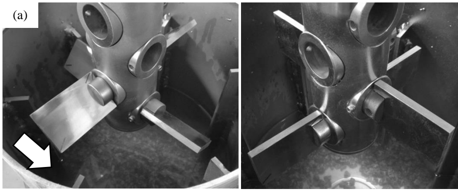
Fig. 2 Sample arrangements with a) +45° (the arrow indicates the direction of rotation) and b) 90° sample angle
