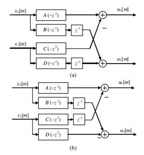
Figure 8. Implementation structure for quadruplets under consideration. (a) Type 1. (b) Type 2.
