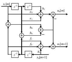
Figure 10. Proposed Implementation structure for one Type 2 quadruplet that is part of a filterbank with *M*=8 and *N*=33.
