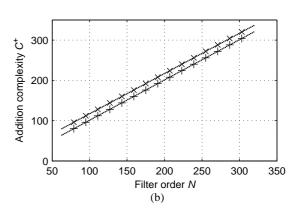
Figure 12. Implementation complexity for filterbanks shown in Figure 11
