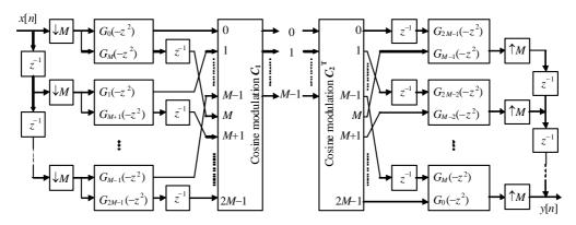
Figure 2. Polyphase structure for implementing a cosine-modulated filterbank.
