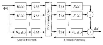
Figure 1. M-channel critically-sampled filterbank.
