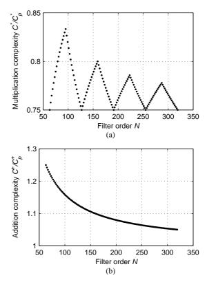
Figure 13. Relative comparison between the proposed method and the polyphase method. (a) Multiplication complexity. (b) Addition complexity.
