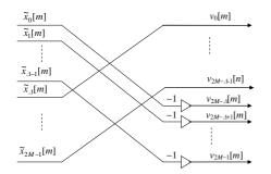
Figure 5. Implementation of the cross-connection matrix  $S_{A}^{(2M)}$ .
