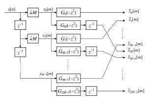
Figure 4. Polyphase implementation of the prototype filter.
