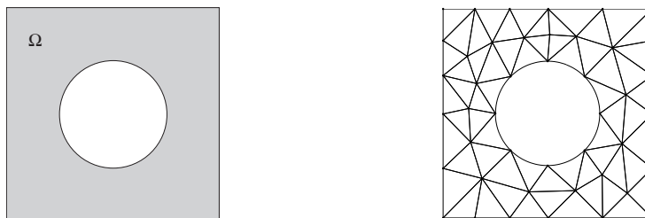
Figure 4: Physical domain with part of the boundary defined by a circular NURBS curve (left) and a valid triangulation for the NEFEM (right)
