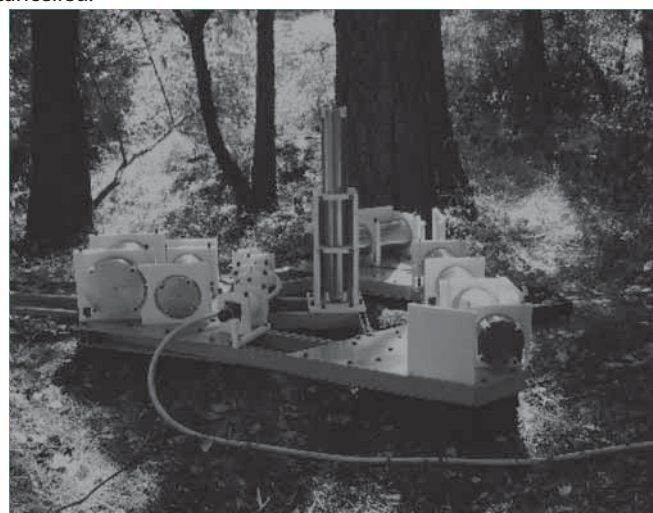
Figure 1. SGO being calibrated against land observatory in Victoria (Canada).
