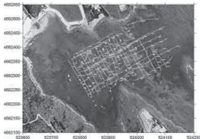
Figure 1: Navigation tracks of the seismo-acoustic records acquired in Port Lligat Bay during the Carbomed Project. Track in red: profile 71 (Fig. 2). Track in yellow: profile 8 (Fig. 3). Red dot: core site
