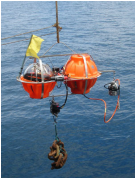
Figure1. Deployment of an Hippocampe OBS from R/V Atalante. The sensor (on the right) will be deployed from the arm when the OBS lay on the sea bottom.
