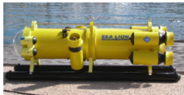
Fig 1. RAO II hull, based on a SeaLion ROV.
