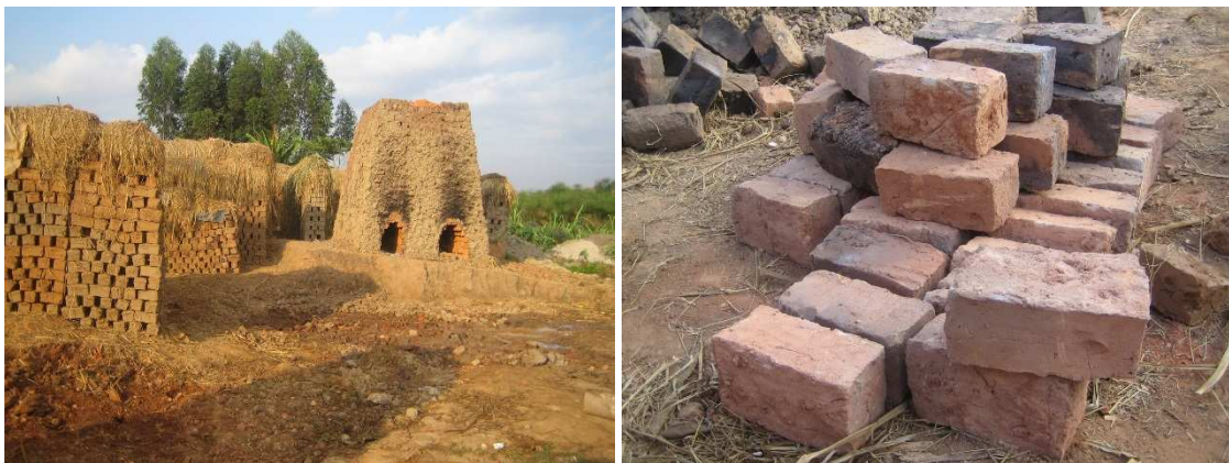
Figure 8. Burned Bricks are very common in both rural and urban areas. Source: The authors.
