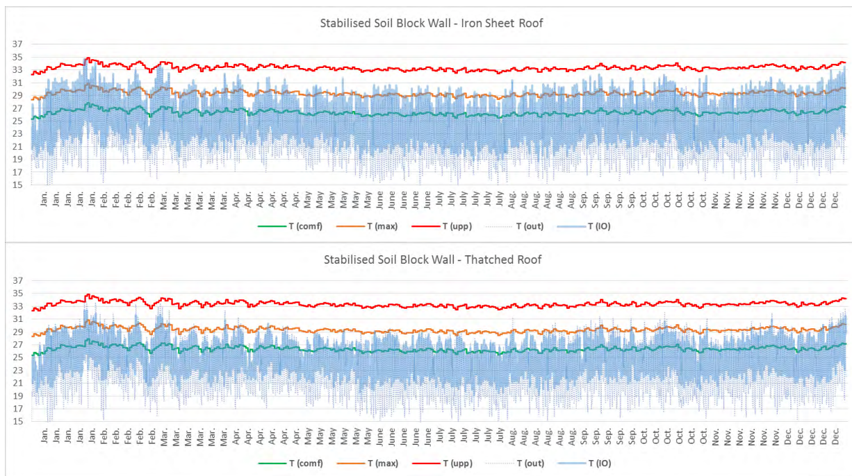
Figure 7: Thermal comfort condition for stabilised soil block walls with iron sheet (top) and thatched roofs (bottom).
