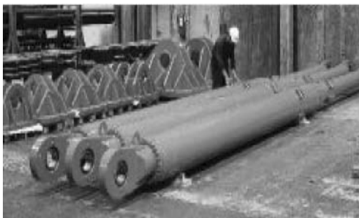
Fig. 1.18 Rion-Antirion Viscous Dampers [Courtesy of FIP Industriale, Italy]
