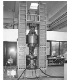
Fig. 2.29 Fuse Element During Fatigue Test [Infanti et al , 2004]
