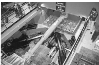
Fig. 2.28 Full-Scale Viscous Damper Prototype Testing [Infanti et al , 2004]
