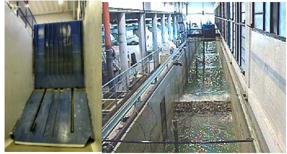
Figure 1: Wave generator(left) and test in progress (right)
