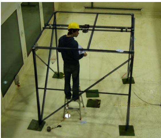
Figure 18: Mooring tests frame
