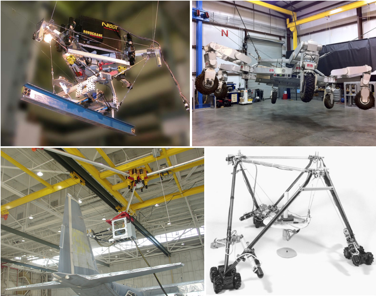
Figure 1: Applications of cable-driven hexapods. From left to right, and top to bottom: Beam manipulation at the NIST Intelligent and Automated Construction Testbed, the ATHLETE Low-gravity Testbed at the Jet Propulsion Lab, fuselage depainting at the NIST Aircraft Maintenance Platform, and a mobile hexapod for oil-well fire fighting.
