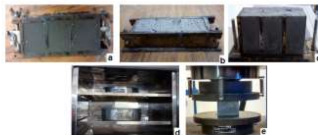
Figure 1. Experiment performed. a) Processing specimens, b) Specimen ready for stripping, c) Unmold specimens, d) Curing chamber, e) Compression test specimens.
