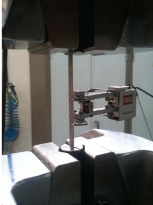
Figure 4 – Experimental tensile test of a corner coupon
