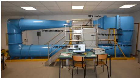
Figure 1: Closed-loop wind-tunnel for backward facing step experiments.
