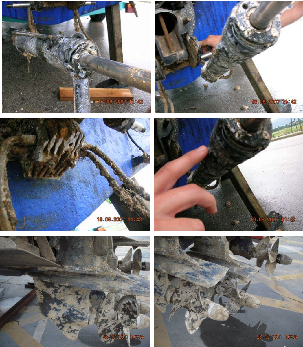
Figure 5 - Serious corrosion in tail propulsion elements (power trim cylinders) and other elements
