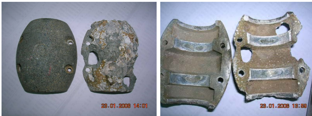
Figure 2 - Zincs defects in the internal contact
