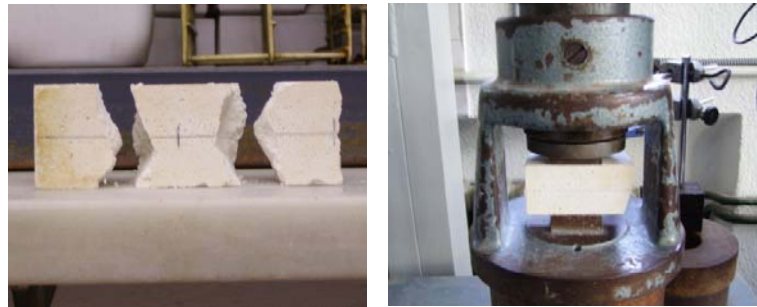
Figure 2. WIKEHAM FARRANCE Sample tested (left). Compressive strength adapter (right)
