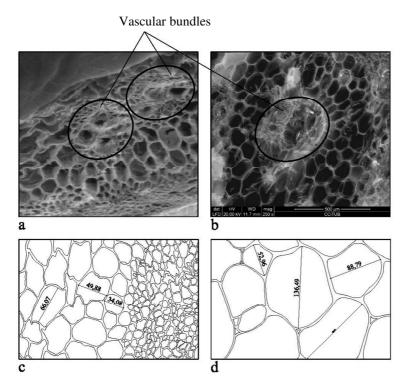
Figure 1. SEM images of barley straw (a) and corn pith (b). Image (a) is scaled four times more than (b). Drawings undernith show both tissues at the same scale, (c) for barley and (d) for corn.
