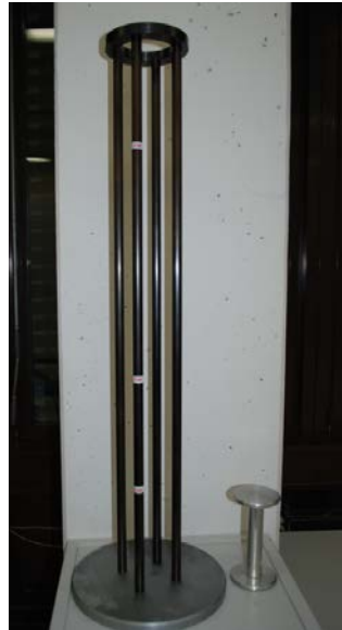
Figure 2-9 Left: loading device for the Essen method for repeated folding and force applications, right: rolling the load device on the looped end [© ELLF]
