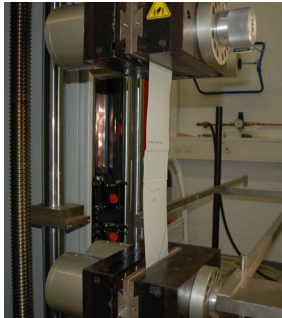
Figure 2-4 Tensile test specimen with welding seam in the testing machine before testing [© ELLF]
