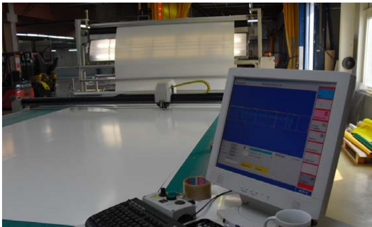
Figure 9-1 Automatically cutting of membrane material via electronic data files [© CENO Membrane Technology GmbH]
