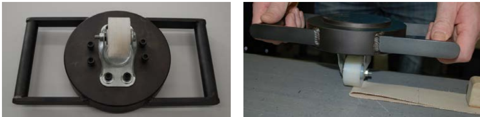
Figure 2-8 Left: loading device for the Essen method for repeated folding and force applications, right: rolling the load device on the looped end [© ELLF]
