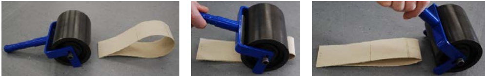
Figure 2-7 Preparation of the looped specimen for the crease fold test acc. to ASTM D4851-07 [© ELLF]
