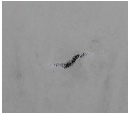
Figure 7-5 "Short cut" in a glass fibre fabric due to previous crease fold [© K. Saxe]
