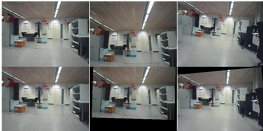
Figure 8 Scene 2. Top: original video. Bottom: stabilized video.
