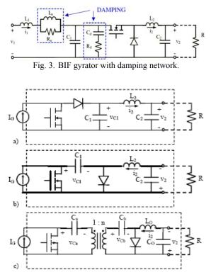
Fig. 4. Classification of *R*-type gyrators: (*a*) boost with output filter (BOF), (*b*) Ćuk converter, and (*c*) Ćuk isolated.
