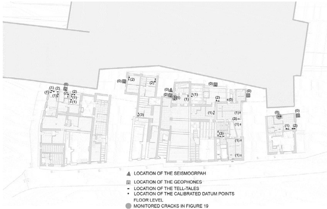
Figure 17: Site plan showing the seismograph, the geophones, the inclinometers, the tell-tales and the calibrated datum points.
