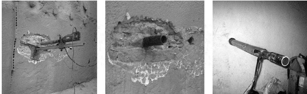
Figure 10: The process of setting up the probe in a Wall of ordinary masonry: Making the hole (left), inserting the probe (centre) and adding pressure (right).
