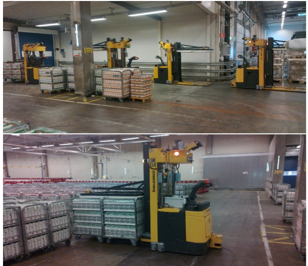
Fig. 1. An example of the real-world application challenges for localization. The dynamics of the environment includes people, moving vehicles, and semi-static layout.
