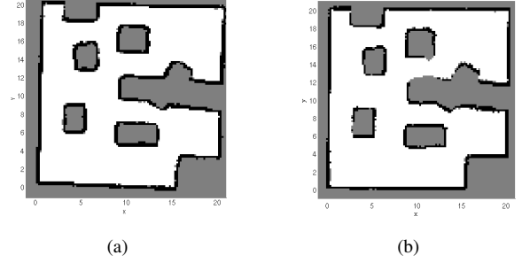
Fig. 4. The final occupancy grid maps; a) exploration with the grid-based method and b) exploration with COM. Inferring the COM with GP regression leads to a partially incomplete equivalent occupancy grid map. See Fig. 5 for a completed experiment with GP regression.
