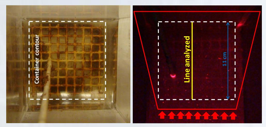
Fig 1. Left: Image of the grid with biosolids. Right: Image obtained indicating the laser projection, the container contour and the line analyzed.
