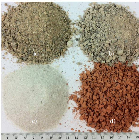
Figure 1. Recycled aggregates: a) NA, b) RCA, c) RGA y d) CRA.
