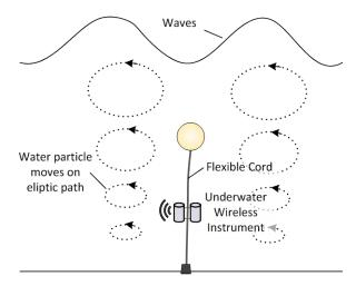
Figure 2 Underwater wireless instruments dynamics in water circular motion induced by waves.
