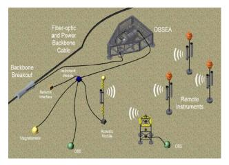
Figure 1 Diagram of underwater observatory. Shows hybrid communication system, measurement equipment with wireless and wired access in underwater environment
