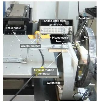
Figure 5 Illustration of the prototype energy harvesting device mounted on a cylinder attached to the shake table, showing the pendulum with the plectra's, the piezoelectric beam, the accelerometer and the gyroscope
