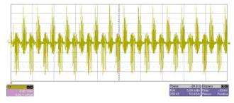
Figure 7 Output voltage of a single piezoelctric plotted versus time for a rotation of the harvesting device of 25 rad/s at 0.33 Hz and with several plectra with 5 mm gap
