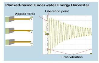
Figure 3 Plucked-driven vibration energy harvester
