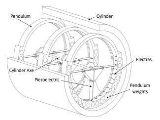
Figure 4 Schematic representation of the proposed underwater energy harvesting systems having three pendulums with three piezoelectric elements for each pendulum
