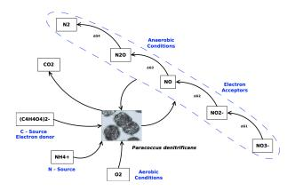
Fig. 1 Schematic representation of INDISIM-Paracoccus model shows the electron donor (Csource), ammonium as N-source and, the different electron acceptors, interacting with the microorganism, which execute their metabolic pathways to obtain denitrification products.
