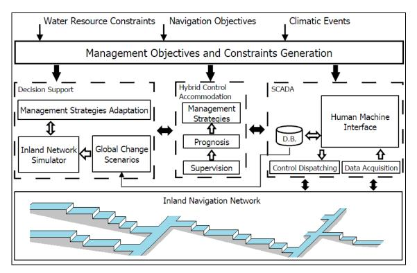
Figure 1- Inland navigation network adaptive and predictive control architecture.
