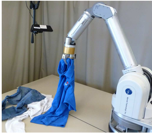
Figure 4: Setup used to acquire the dataset. Garments lay on the table in different positions and deformations. RGB-D images are acquired using a Kinect camera looking downwards on a WAM robot cell.
