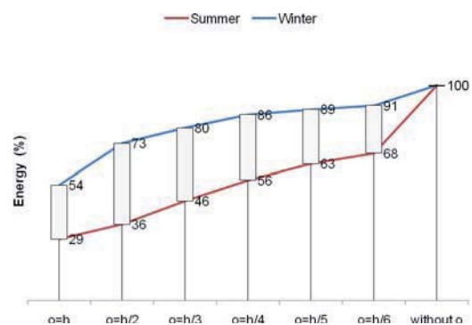
Figure 6: percentage of radiation received with different lengths of overhangs, in Barcelona, in summer and winter
