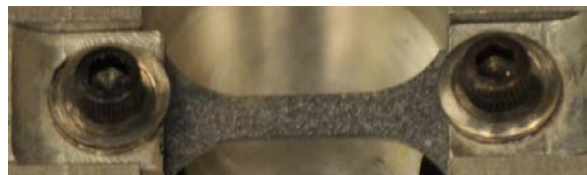
Figure 6. Black and white speckle pattern applied to the coupon outer surface.
