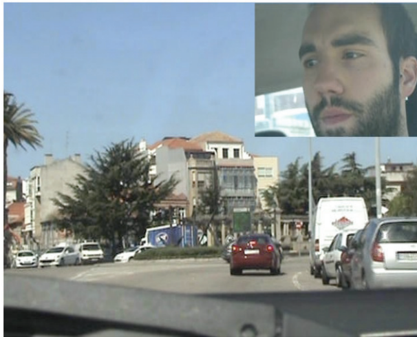
FIGURE 1 Video stream showing the face of the driver (to assess blinking and saccades) and the scene as observed through the windshield of the car (to determine driving complexity).
