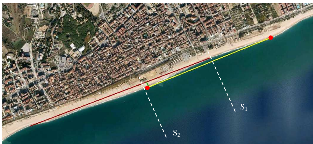
Figure 3. Plan view of the beach of Calella. Red circles indicate two consecutive salients along Calella beach with a spacing of 1240 m. The cross-shore displacement of the tip of the salients with respect to the embayments (amplitude) is a_s \approx 48 m.
