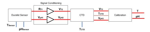
Figure 2 Description of the measurement system
