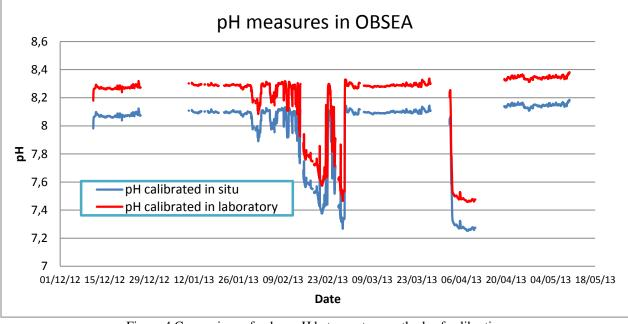
Figure 4 Comparison of values pH between two methods of calibration
