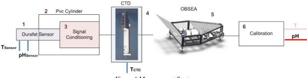
Figure 1 Measurement System
