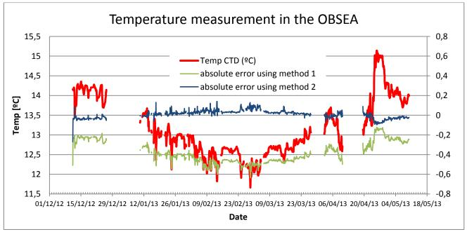
Figure 3 Comparison of values temperature between two methods of calibration
