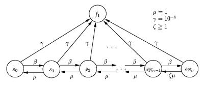
Figure 7. State transition diagram of the paradigmatic CTMC.
