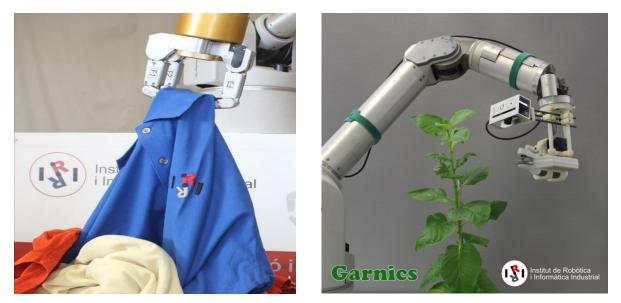
Setups for some projects on robot perception and manipulation recently developed at IRI (CSIC-UPC): a) perceiving and handling clothes [7, 8], b) measuring the chlorophyll of plant leaves for phenotyping [2].
