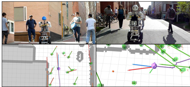
Fig. 6. Real experiments. Top: some pictures of the social-aware navigating in the BRL. Bottom: their corresponding sensor information and relevant information in the robot GUI.
