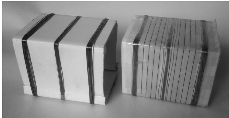
Figure 2. Prismatic inductors of 6 cm side. Designed with analytical method (left) and trial-and-error (right).
