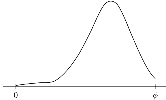
Figure 6.22. Estimated force distribution over disc cutter.
