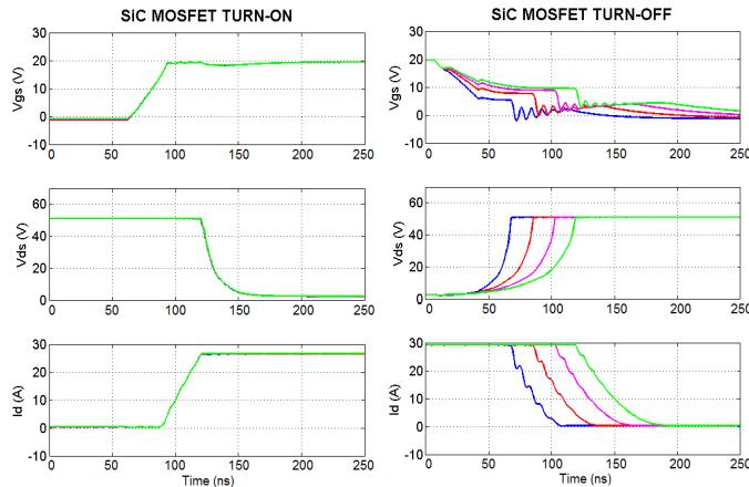
Fig. 15. Effect of parallel RD coupling circuit on switching characteristics (simulated results). Cases:  $R_{toff} = 0\Omega$  (blue trace),  $R_{toff} = 5\Omega$  (red trace),  $R_{toff} = 10\Omega$  (pink trace) and  $R_{toff} = 15\Omega$  (green trace).
