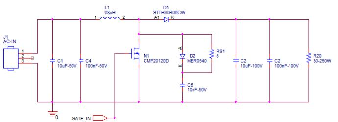
Fig. 1. Schematic of the boost converter.
