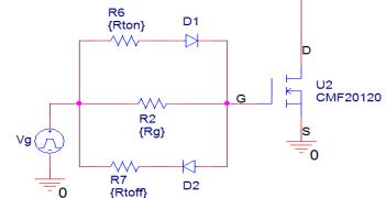
Fig. 4. Parallel RD (Resistance Diode) coupling circuit
