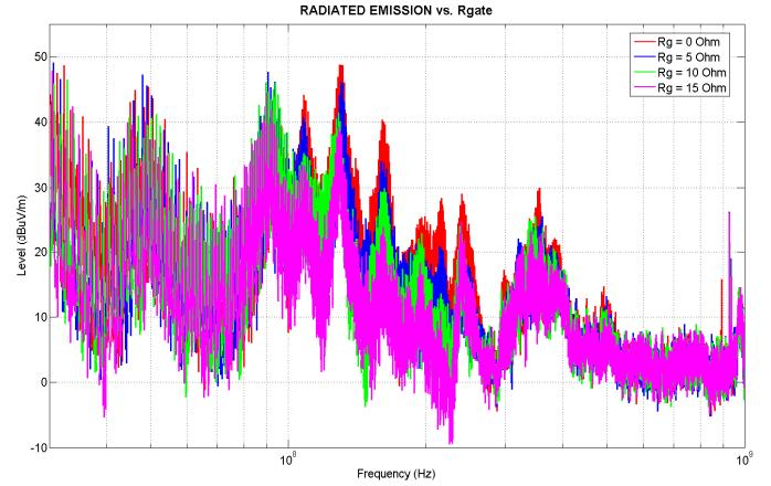
Fig. 8. Effect of the series resistor on radiated EMI (experimental results). Cases:  $R_g = 0 \Omega$  (red trace),  $R_g = 5 \Omega$  (blue trace),  $R_g = 10 \Omega$  (green trace) and  $R_g = 15 \Omega$  (pink trace).
