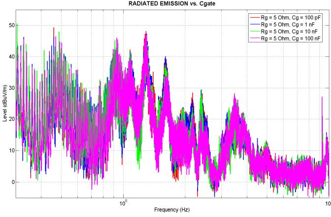
Fig. 14. Effect of RC coupling circuit on radiated emissions (experimental results). Cases:  $C_g = 100\text{ pF}$  (red trace),  $C_g = 1\text{ nF}$  (blue trace),  $C_g = 10\text{ nF}$  (green trace),  $C_g = 100\text{ nF}$  (pink trace).
