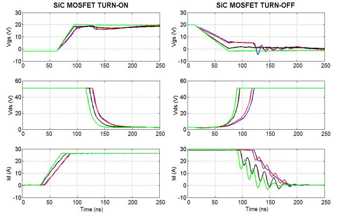
Fig. 12. Effect of RC coupling circuit on switching characteristics (simulated results). Cases:  $C_g = 100\text{ pF}$  (green trace),  $C_g = 1\text{ nF}$  (black trace),  $C_g = 10\text{ nF}$  (red trace),  $C_g = 100\text{ nF}$  (blue trace).
