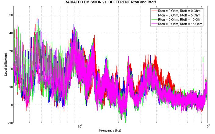
Fig. 17. Effect of parallel RD coupling circuit on radiated EMI (experimental results). Cases:  $R_{ton} = 0\Omega$ ,  $R_{toff} = 0\Omega$  (blue trace),  $R_{ton} = 0\Omega$ ,  $R_{toff} = 5\Omega$  (red trace),  $R_{ton} = 0\Omega$ ,  $R_{toff} = 10\Omega$  (pink trace) and  $R_{ton} = 0\Omega$ ,  $R_{toff} = 15\Omega$  (green trace).
