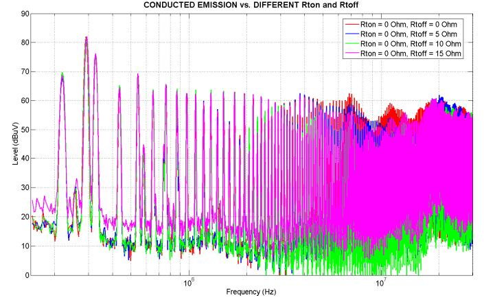
Fig. 16. Effect of parallel RD coupling circuit on conducted EMI (experimental results). Cases:  $R_{ton} = 0\Omega$ ,  $R_{toff} = 0\Omega$  (blue trace),  $R_{ton} = 0\Omega$ ,  $R_{toff} = 5\Omega$  (red trace),  $R_{ton} = 0\Omega$ ,  $R_{toff} = 10\Omega$  (pink trace) and  $R_{ton} = 0\Omega$ ,  $R_{toff} = 15\Omega$  (green trace).
