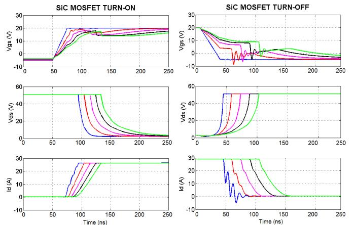
Fig. 5. Effect of the series gate resistor on switching characteristics (simulation results). Cases:  $R_g = 0 \Omega$  (blue trace),  $R_g = 5 \Omega$  (red trace),  $R_g = 10 \Omega$  (pink trace),  $R_g = 15 \Omega$  (black trace) and  $R_g = 20 \Omega$  (green trace).
