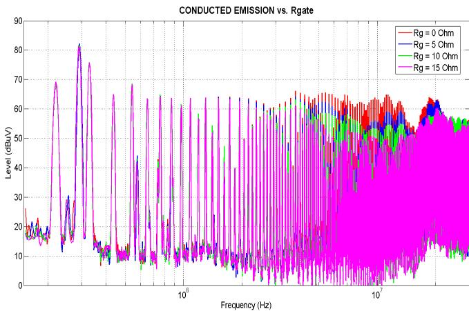
Fig. 7. Effect of the series resistor on conducted EMI (experimental results). Cases:  $R_g = 0 \Omega$  (red trace),  $R_g = 5 \Omega$  (blue trace),  $R_g = 10 \Omega$  (green trace) and  $R_g = 15 \Omega$  (pink trace) were used.
