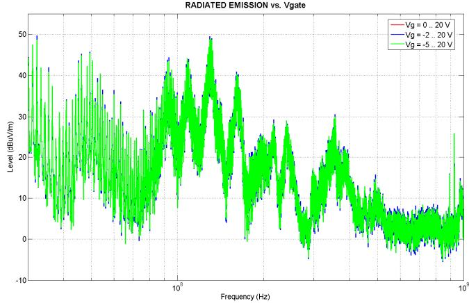
Fig. 11. Effect of the gate voltage on radiated EMI (experimental results). Cases:  $V_g = 0$  to 20 V (blue trace),  $V_g = -2$  to 20 V (red trace) and  $V_g = -5$  to 20 V (green trace).
