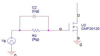
Fig. 3. Parallel RC coupling circuit.
