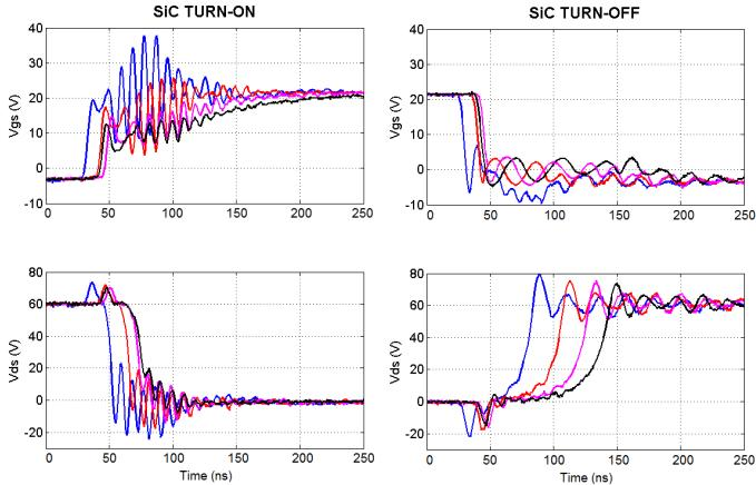
Fig. 6. Effect of the series gate resistor on switching characteristics (experimental results). Cases:  $R_g = 0 \Omega$  (blue trace),  $R_g = 5 \Omega$  (red trace),  $R_g = 10 \Omega$  (pink trace) and  $R_g = 15 \Omega$  (black trace).
