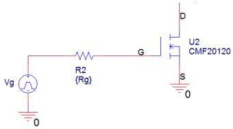
Fig. 2. Driver to gate coupling resistor.
