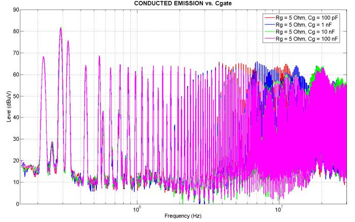
Fig. 13. Effect of RC coupling circuit on conducted EMI (experimental results). Cases:  $C_g = 100\text{ pF}$  (red trace),  $C_g = 1\text{ nF}$  (blue trace),  $C_g = 10\text{ nF}$  (green trace),  $C_g = 100\text{ nF}$  (pink trace).
