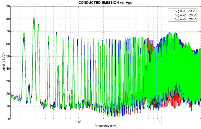
Fig. 10. Effect of the gate voltage on conducted EMI (experimental results). Cases:  $V_g = 0$  to 20 V (blue trace),  $V_g = -2$  to 20 V (red trace) and  $V_g = -5$  to 20V (green trace).
