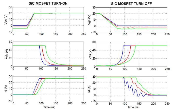
Fig. 9. Effect of the gate voltage on switching characteristics (simulation results). Cases:  $V_g = 0$  V to  $20$  V (blue trace),  $V_g = -2$  V to  $20$  V (red trace) and  $V_g = -5$  V to  $20$  V (green trace).
