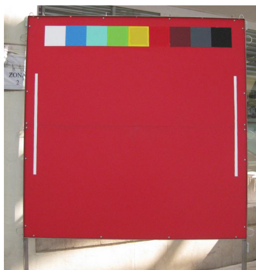
Figure 2. The methacrylate red panel used for automated RGB colorimetric calibration of images taken by OBSEA camera at different times of the day. White vertical lines (100 cm length) can be used as general size bars for fish length determination in absence of more precise measuring methods ( i.e. , lasers).
