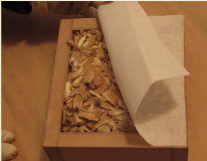
Insulation made of filters of cigarettes
