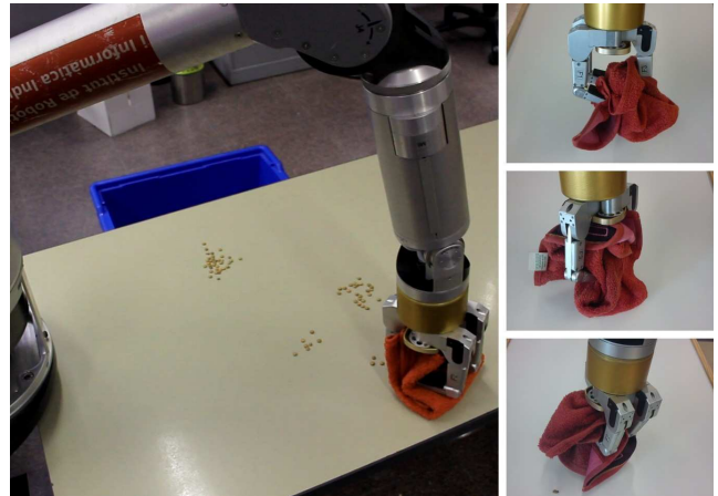
Figure 1: On the left the WAM robot arm is cleaning lentils from a table to a container. On the right three different grasps of the textile used for cleaning, each one leading to different behaviours of the cleaning actions.
