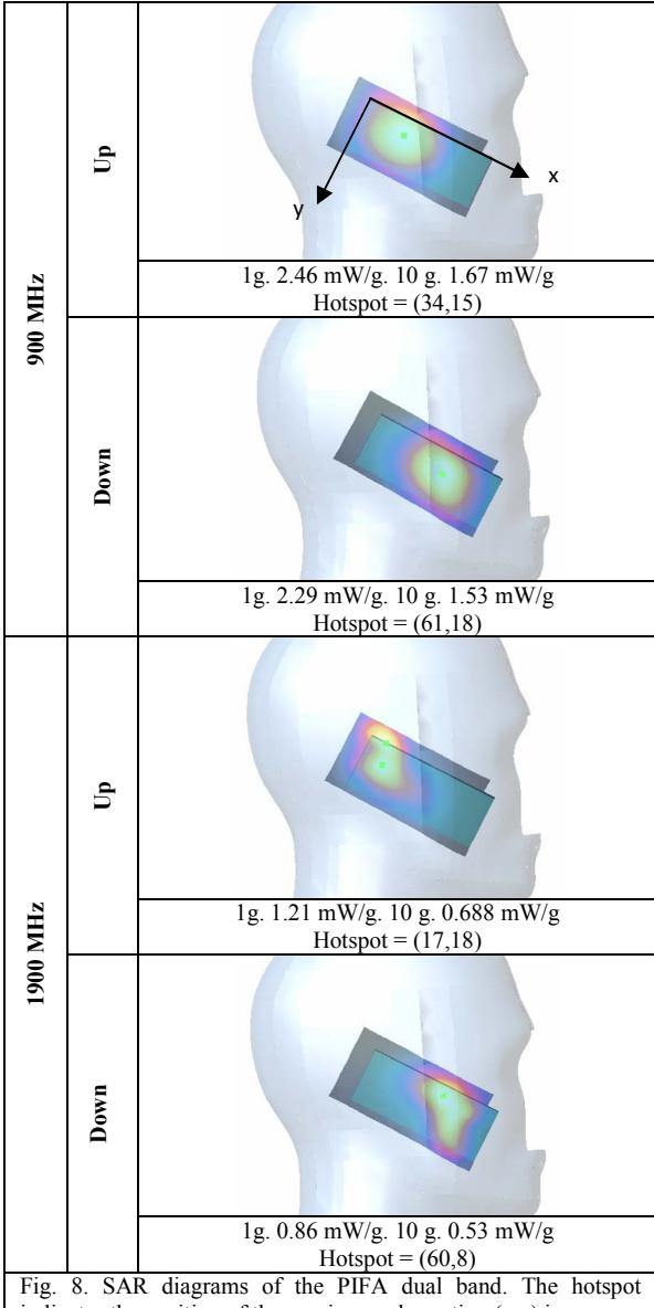
At 900 MHz, SAR values do not differ from up and down position (Table II). In all the antennas, the hotspot is situated approximately in the middle of the ground plane because at
