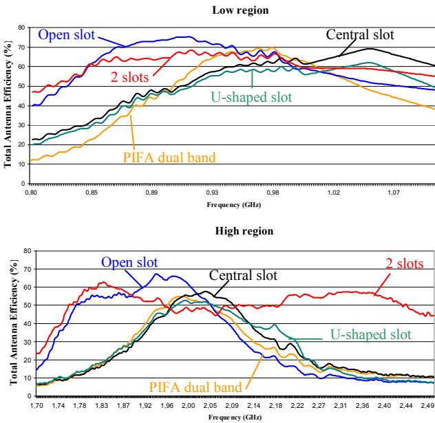
Fig. 5. Measurements of the Total Antenna Efficiency at low and high region
