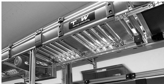
Fig. 2. An example of a roller conveyor similar to that modeled in the project (Source Wikipedia)
