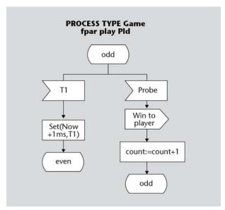
Figure 8. Specification and Description Language process detailing a simulation model behavior
