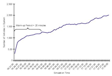
Figure 11. Determining the warm-up period through a time series
