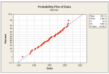
Figure 9. A Q-Q plot for testing normality of data
